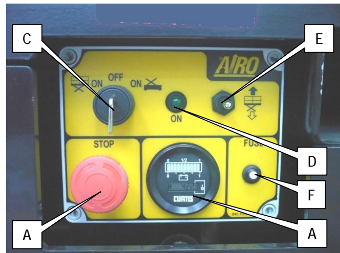
5-3: Ground control panel
