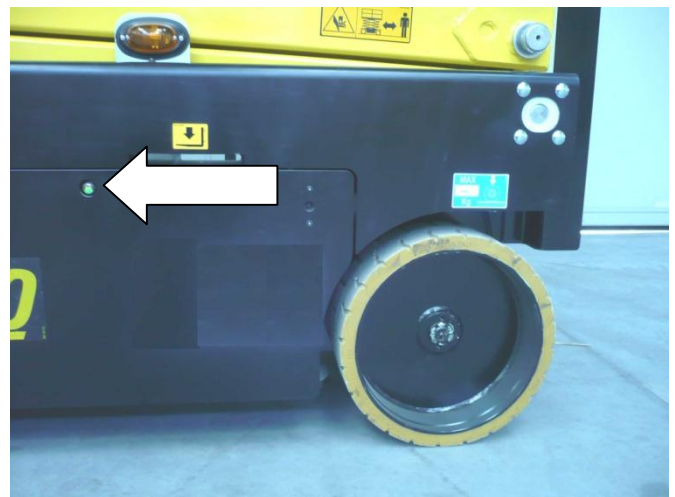
7-14: Battery charger light
