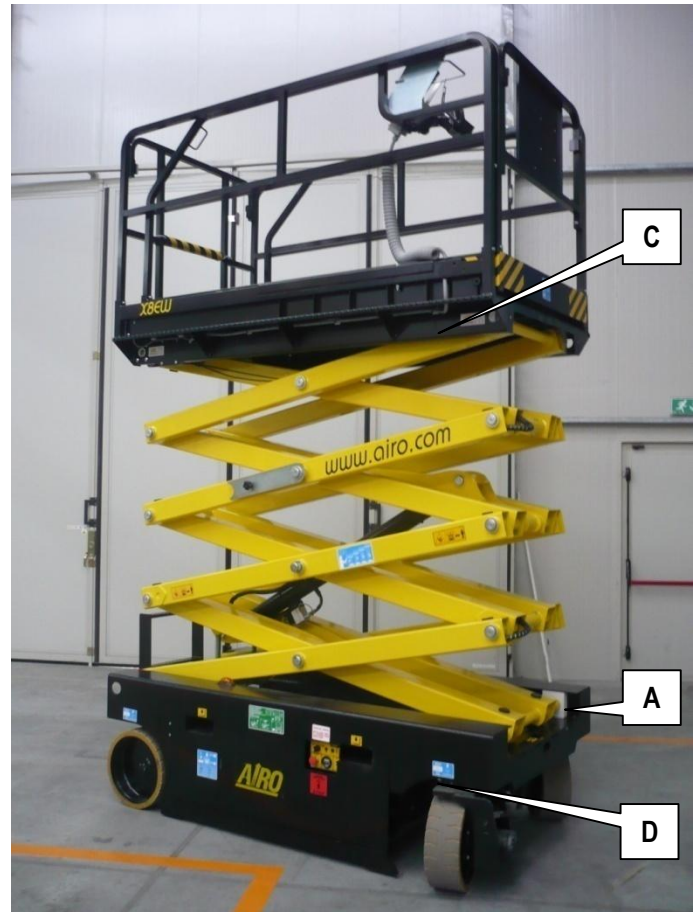
7-5: Location of main parts to be greased
