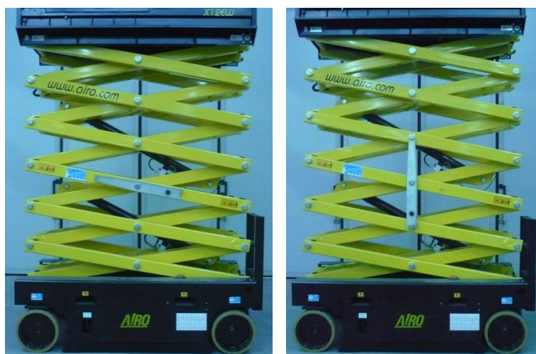
7-3: Saksirakenteen lukitus: X12 EN, X12 EW, X12 EW-WIND, X14 EW, X16 EW, XS9 E RESTYLING
