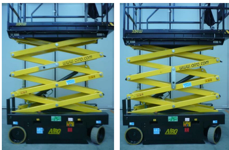
7-2: Saksirakenteen lukitus: X10 EN, X10 EW, X10 EW-WIND, XS8 E RESTYLING LIGHT, XS8 E RESTYLING
